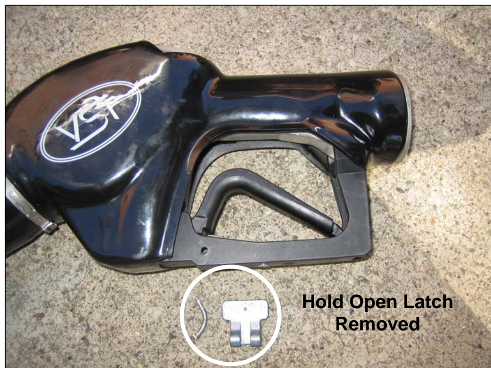
Figure 2: VST Balance Nozzle with Hold Open Latch Removed
